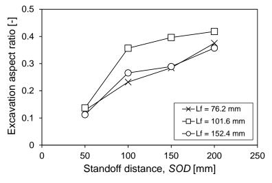
Fig. 4 Effect of standoff distance and focusing tube length on the excavation aspect ratio
